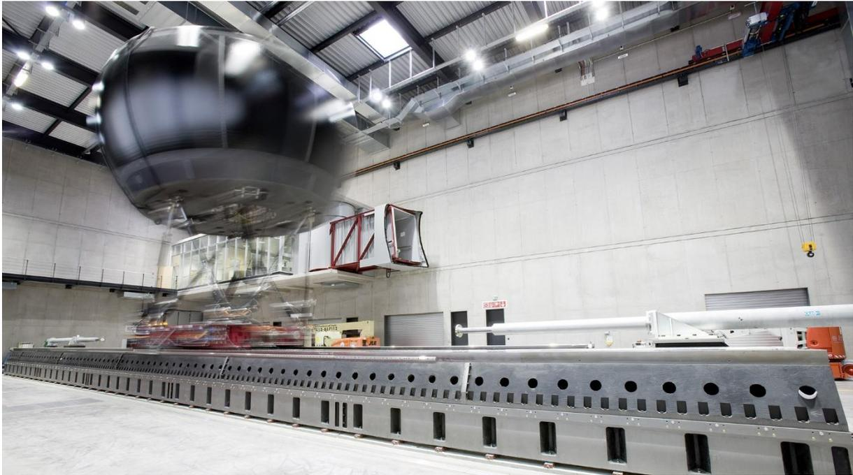
**Caption: Driving simulator installed at Daimler AG in Sindelfingen, Germany. The mechanical parts of the system except the Hexapod have been designed and installed by Imtec Engineering (image courtesy of Daimler AG)**
