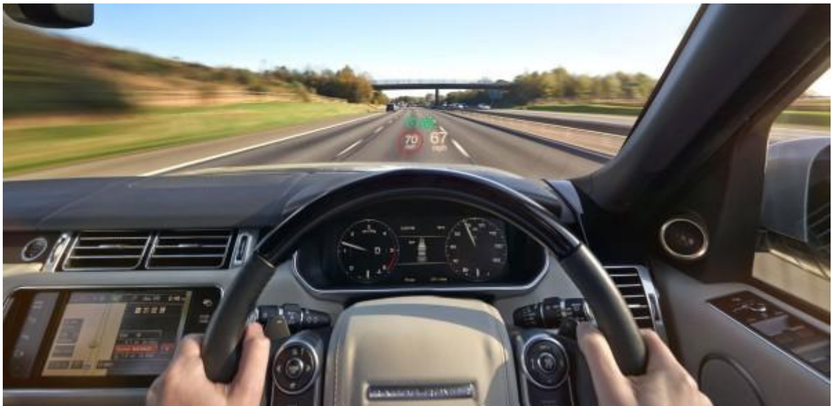
Fig. 4.2. A head-up display for passenger vehicles developed at Cambridge, the first to incorporate holographic techniques, has been incorporated into Jaguar Land Rover vehicles.
